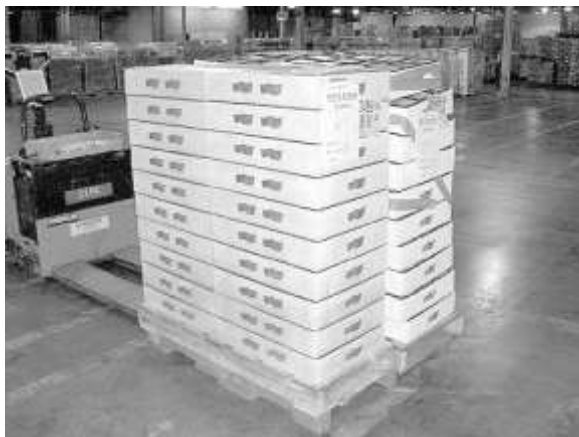
Figure 4-19 – Improperly Piled Half Pallet
